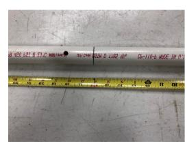
2. Slide the top portion of the 30" piece of 1" PVC pipe into one end of the 1 1/4" PVC pipe and stop at the line previously drawn marking the 16" mark on the 30" pipe. Drill 1 or 2 holes through the two layers of PVC pipe approximately 12 inches apart using a 5/16" drill bit. Then fasten the two pipes together with one of the locking pins.
